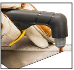
• Use a metal straight edge to control cuts
