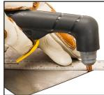
• Use a metal straight edge to control cuts
