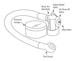
The air hose, pressure gauge and brass air manifold set are assembled on the tank by the factory. Please inspect for any loose fittings or bolts before putting into service.
